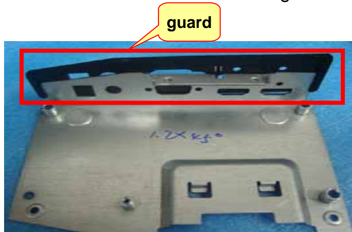
S6: Assemble the chassis and a guard.
